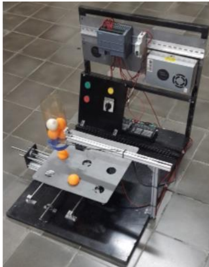
Figure 6. Object Placement System Based on Siemens S7-1200
